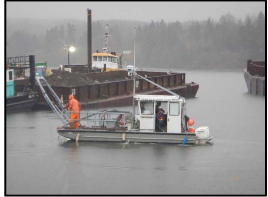
Confirmatory sediment cores being collected.
